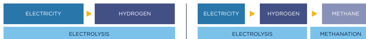
Figure 3: Power2Gas concepts: Power2Hydrogen and Power2Methane 53
